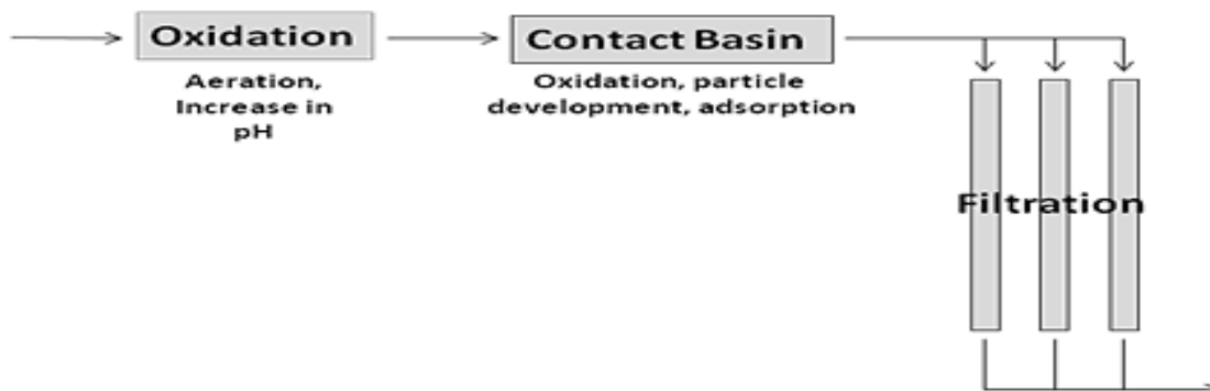
FIG. 2. Schematic diagram of removal of Fe, As and Mn from water.
