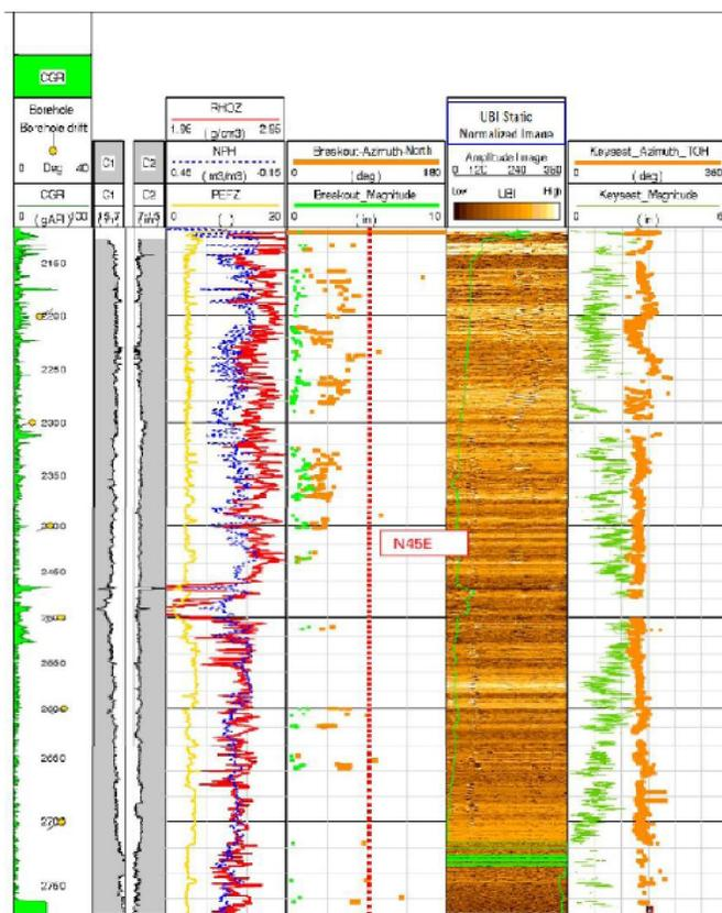
Figure 8 : In well GS-D, the composite plot of calipers and full set logs showing the borehole breakout and key seat azimuths and magnitudes which were derived from UBI images. The average breakout azimuth is N45E for the intervals with well deviation less than 20 degrees. Breakout azimuths in intervals with inclination higher than 20 degrees do not represent the exact orientation of breakouts. In such cases, breakout orientations need to be corrected
