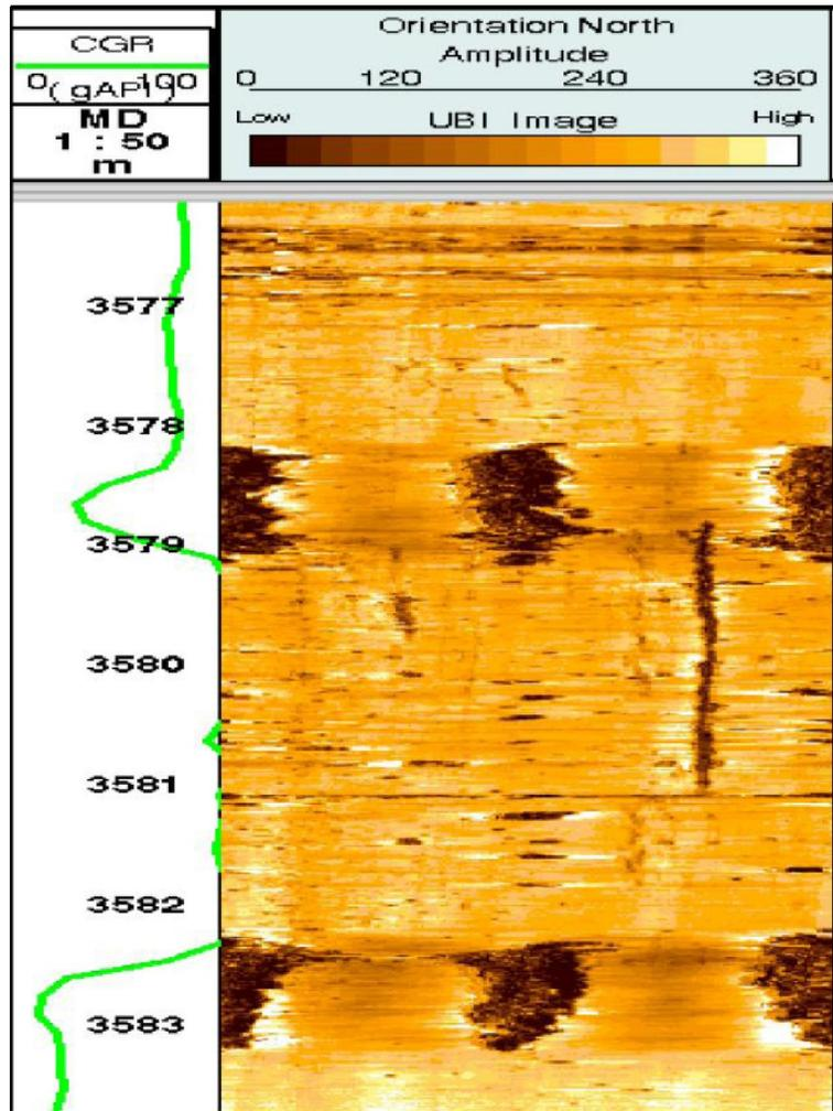
Figure 3 : The UBI image showing borehole breakouts and drilling induced fractures; the thin dark color region is drilling induced fracture, and the dark wide regions are borehole breakouts
