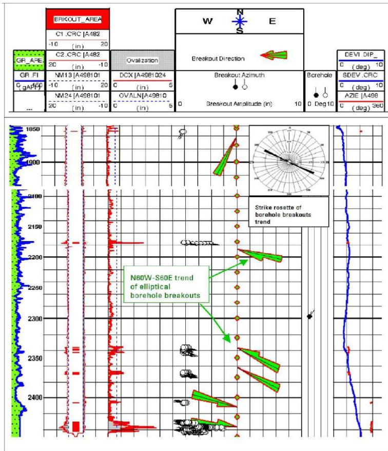
Figure 13 : In well GS-F, the logs showing dominantly N60W-S60E trending for borehole breakouts in Asmari formation. The breakouts were mostly observed in lower section. According to them the orientation of  $\sigma_{hmin}$  is N60W-S60E and the orientation of  $\sigma_{hmax}$  is N30E-S30W
