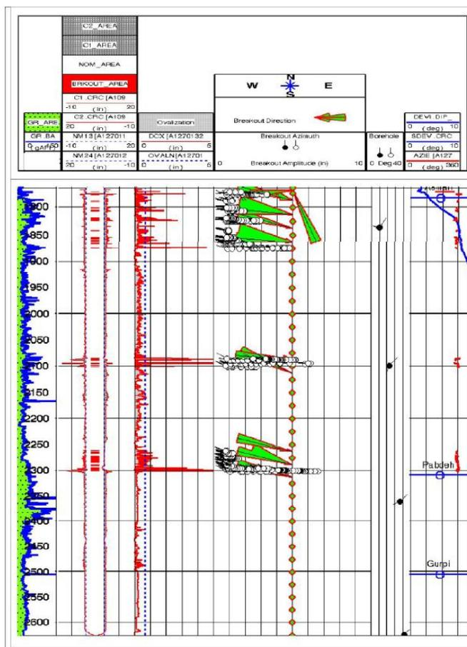
Figure 15 : In well GS-G, the logs showing the WNW-ESE trend for borehole breakouts in the Asmari formation. According to them the orientation of  $\sigma_{hmin}$  is WNW-ESE and the orientation of  $\sigma_{hmax}$  is NNE-SSW
