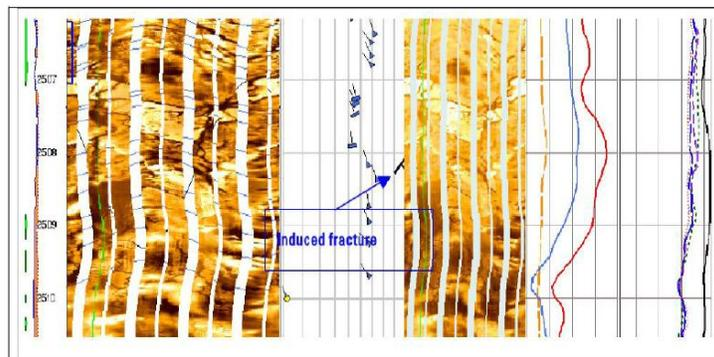
Figure 10 : In the well GS-E images shows the NE-SW trend for the drilling induced fractures in depth 2508m; header is given in Figure 9
