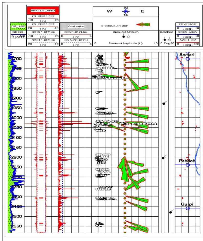
Figure 17 : In well GS-H, the logs showing E-W trend for the borehole breakouts in the Asmari formation and the NW-SE trend in the Pabdeh and Gurpi formations. The breakouts were mostly observed in the Pabdeh formation. The borehole trend in Pabdeh formation is slightly different from the Asmari formation. According to them the overall orientation of  $\sigma_{hmin}$  is N57W-S57E and the orientation of  $\sigma_{hmax}$  is N33E-S33W
