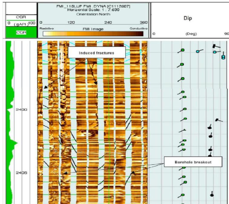
Figure 14 : In well GS-G, FMI images showing induced fractures in the upper part of the figure (2395m-2402m) and borehole breakouts in lower part (2402m-2407m). They have 90 degrees difference in the azimuth
