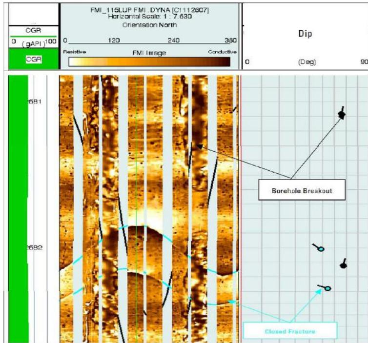
Figure 5 : In well GS-A, the FMI images showing borehole breakouts on the images
