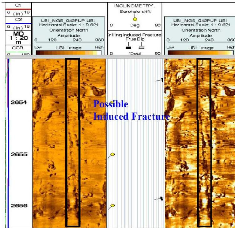
Figure 18 : The UBI image showing drilling induced fractures in the wellGS-I
