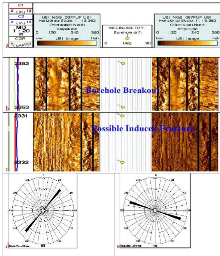
Figure 6 : a) UBI log header in well GS-B; b & c) UBI images show borehole breakouts striking almost NE-SW, which is parallel to  $\sigma_{hmin}$ , and the orientation of the drilling induced fractures that is WNW-ESE to be parallel to  $\sigma_{hmax}$  orientation; d) strike of  $\sigma_{hmin}$  in Schmidt projection & e) strike of  $\sigma_{hmax}$  in Schmidt projection
