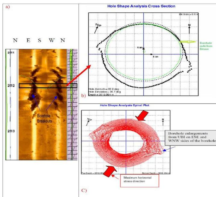
Figure 7 : a) In well GS-C, the UBI image of the borehole radius showing borehole enlargements (breakouts – black vertical stripes) around WNW and ESE sides of the borehole in the well GS-C; b) and c) The pipe’s down-looking view of the borehole radii from the UBI
