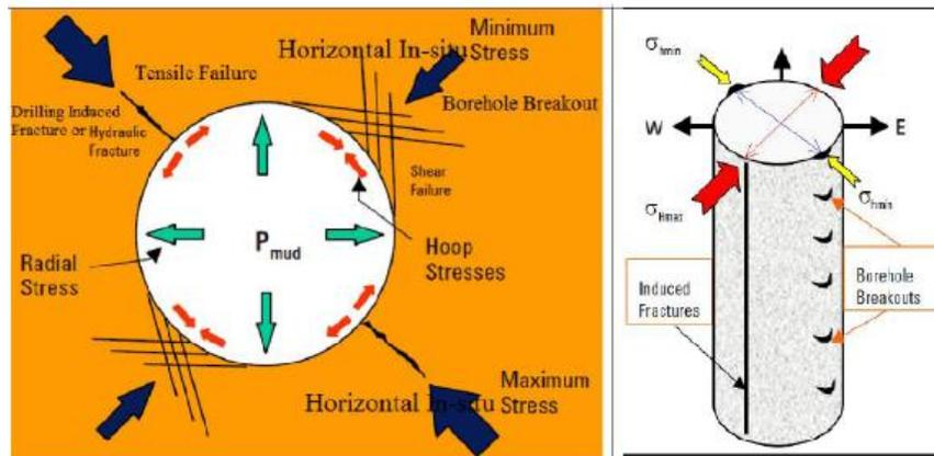
Figure 4 : schematic pictures of the radial stress, tensile failure, drilling induced fracture (hydraulic fracture), maximum horizontal stress, hoop stress, shear failure, borehole breakout and minimum horizontal stress
