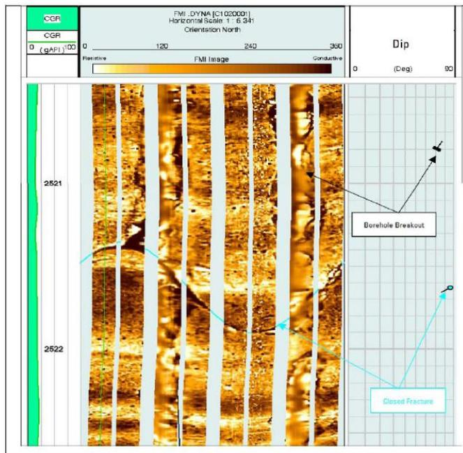
Figure 16 : In well GS-H, the FMI images showing borehole breakouts on the images facing northwest (N57W to be more precise) and southeast (S57E to be more precise) sides of the borehole. Thus they indicate N57W-S57E trending elliptical borehole breakouts that are aligned with  $\sigma_{hmin}$
