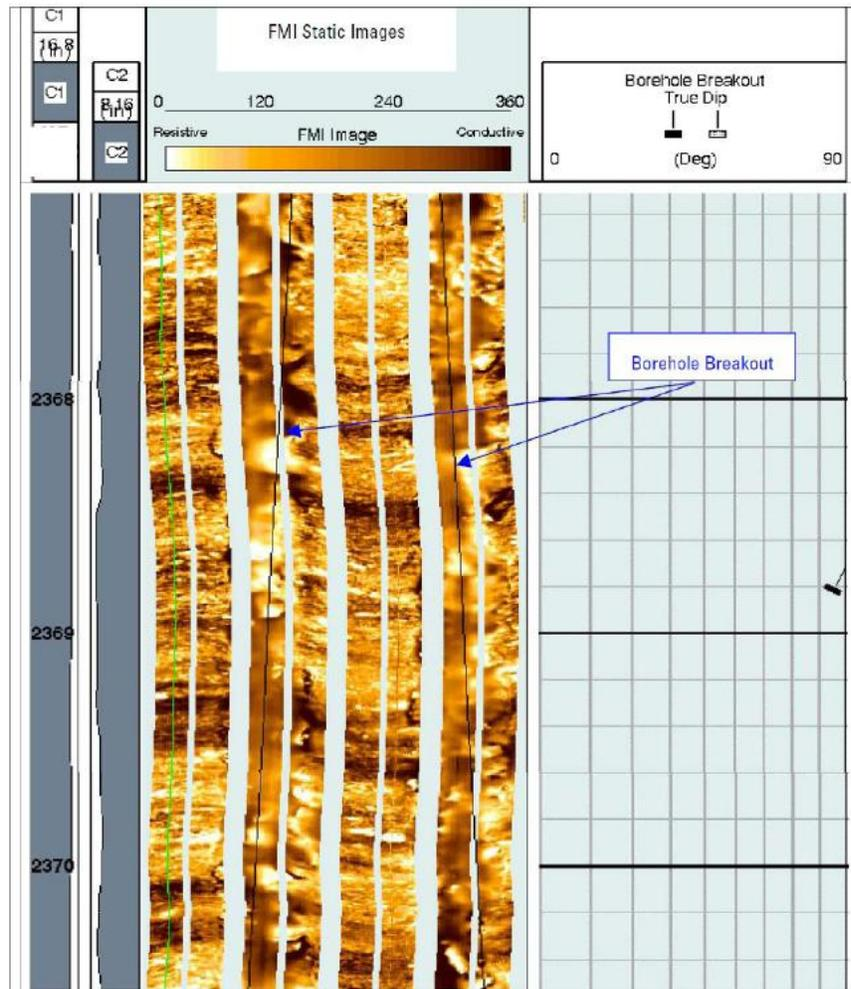
Figure 12 : In the well GS-F, the FMI images showing borehole breakouts on the images facing northwest (N60W to be more precise) and southeast (S60E to be more precise) sides of the borehole. Thus they indicate N60W-S60E trending for  $\sigma_{\text{hmin}}$
