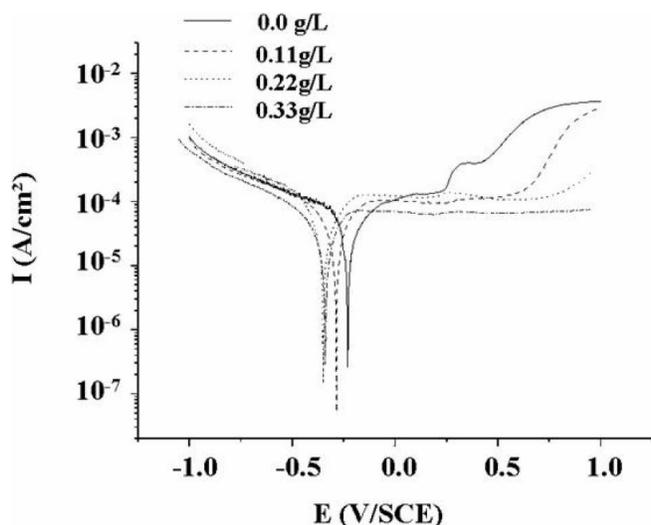
Figure 3 : Polarization curves of dental amalgam alloy in synthetic saliva media at  $37 \pm 1$  °C containing different concentration of anise extract of Morocco.
