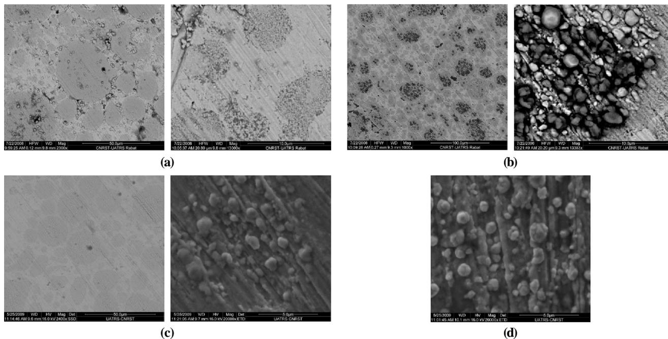
Figure 4 : SEM micrographs of the surface of dental amalgam alloy before and after immersion in synthetic saliva media : (a) before immersion; after immersion (b) in the absence of inhibitor (c) in presence of "anise extract of Yemen (d) in presence of "anise extract of Morocco.
