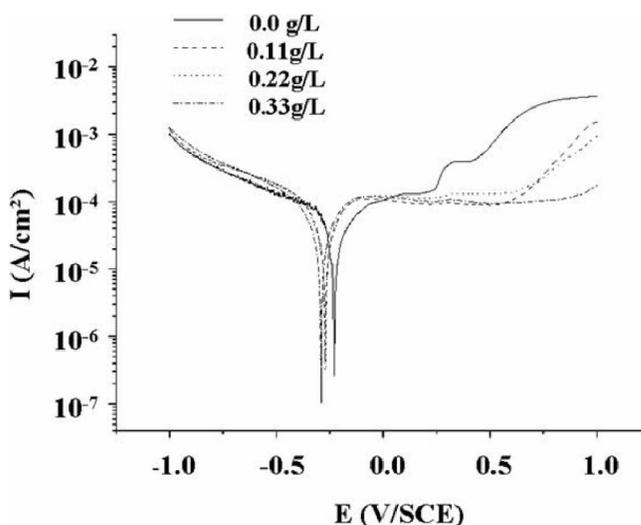
Figure 2 : Polarization curves of dental amalgam alloy in synthetic saliva media at 37 ± 1 °C containing different concentration of anise extract of Yemen.
