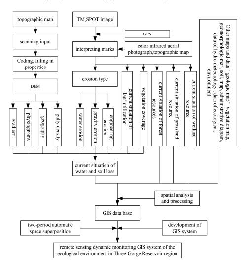
Figure 1 : Remote sensing dynamic monitoring process of ecological environment
