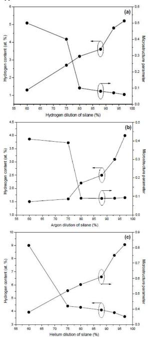
Figure 4: Variation of hydrogen content ( $C_H$ ) and microstructure parameter ( $R^*$ ) as a function of dilution of silane using different diluents for the nc-Si:H deposited thin films by HW-CVD.
