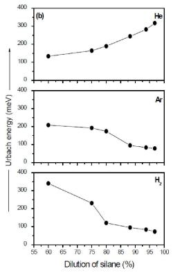
Figure 5: Variation of band gap and Urbach energy as a function of dilution of silane using different diluents for the nc-Si:H deposited thin films by HW-CVD.
