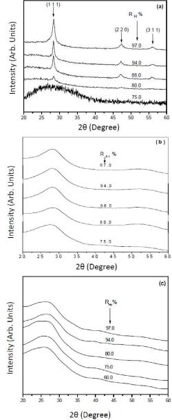
Figure 3: X-ray patterns of films deposited at different dilution of silane using different diluents (a) Hydrogen dilution of silane (b) Argon dilution of silane and (c) Helium dilution of silane.
