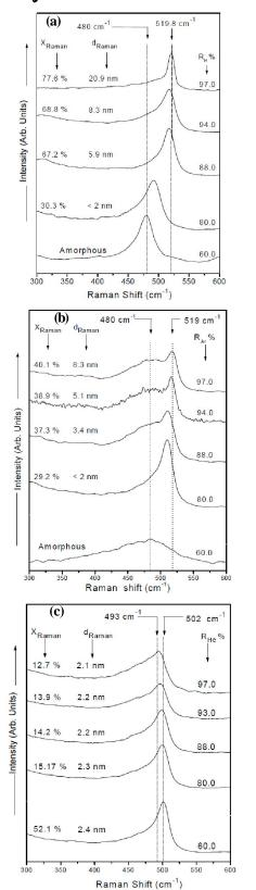
Figure 2: Raman spectra of films deposited at different dilution of silane using different diluents (a) Hydrogen dilution of silane (b) Argon dilution of silane and (c) Helium dilution of silane.
