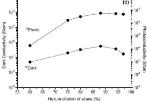
Figure 6: Variation of dark and photoconductivity as a function of dilution of silane using different diluents for the nc-Si:H deposited thin films by HW-CVD.
