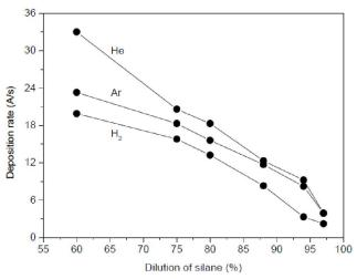
Figure 1: Variation of deposition rate as a function of dilution of silane by H<sub>2</sub>, Ar and He gases.
