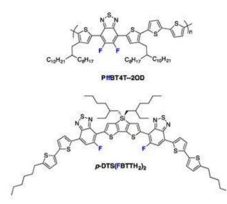
Chemical structures of highly efficient fluorinated materials for organic photovoltaics (OPV)
