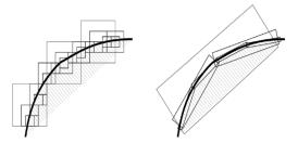
Fig. 2: Wavelets and contourlets in representing a smooth contour
