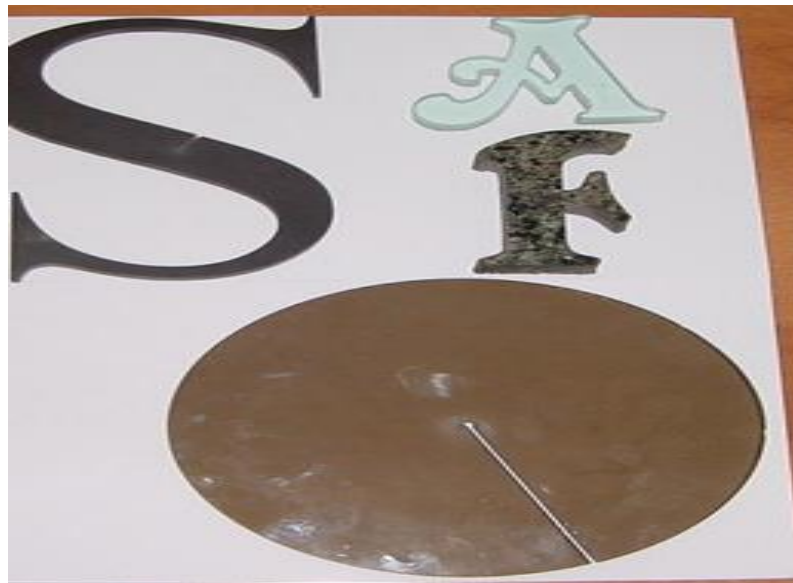
FIG. 2. First high power water cooled porous mirrors.
