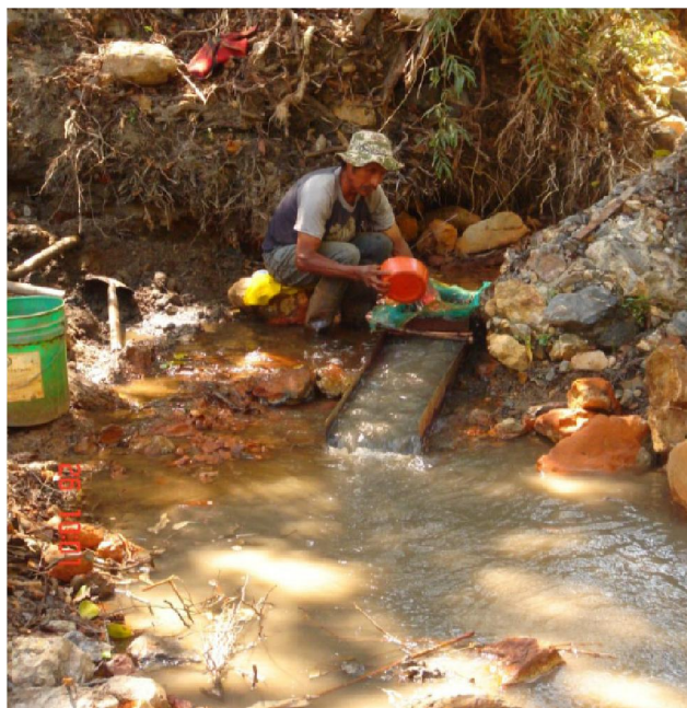
Figure 2 : Gambusino (gold seeker) washing mining tailings to recover the precious metal.
