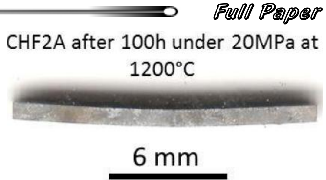
Figure 3 : Illustration of the very good creep-resistance at elevated temperature of one of the HfC-strengthened alloys by the macrograph of a parallelepiped slightly deformed after a 100h-long 3-point central flexural creep test carried out at 1200°C for a 20 MPa resulting maximal tensile stress (office scanner)
