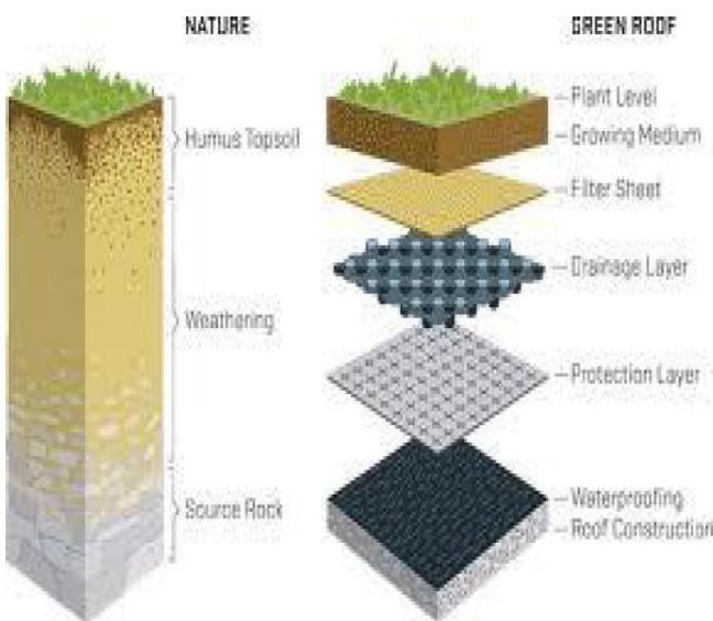
**Figure 2 : Diagrammatic representation of green roof methodology.**
