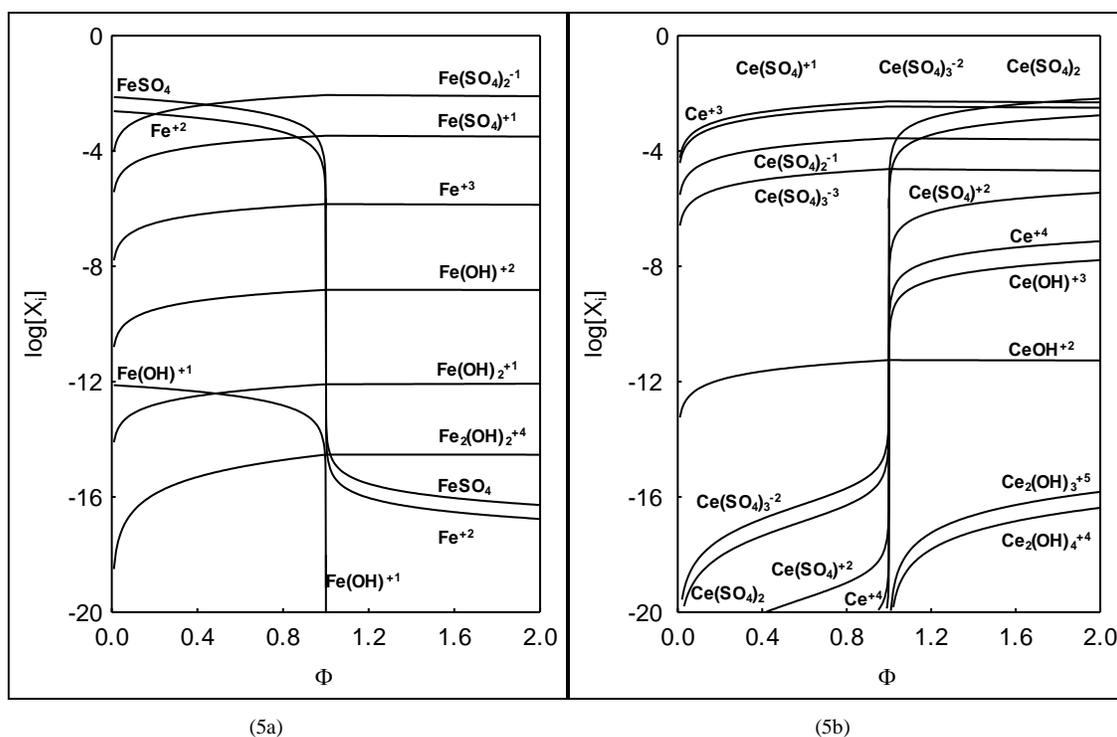
FIG. 5. Speciation curves for (5a) Fe-species and (5b) Ce-species in the system, where  $V_0=100$  mL of  $FeSO_4$  ( $C_0=0.01$  mol/L)+ $H_2SO_4$  ( $C_{01}=1.0$  mol/L) is titrated with  $V$  mL of  $Ce(SO_4)_2$  ( $C=0.1$  mol/L)+ $H_2SO_4$  ( $C_1=0.5$  mol/L) [34].
