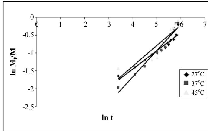
**Fig. 18:** Plot of  $\ln M_t/M_\infty$  vs.  $\ln t$  for release of Cefixime from SCMC beads at pH 1.2, different temperatures, and shaking speed 80 rpm
