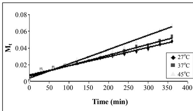
**Fig. 12: Plot of  $M_t$  vs. time of release of cefixime from SCMC beads at pH 1.2, different temperatures, and shaking 80 rpm**
