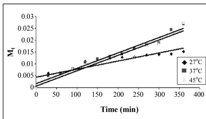
**Fig. 13: Plot of  $M_t$  vs. time of release of Cefixime from SCMC beads at pH 7.2, different temperatures, shaking 80 rpm**
