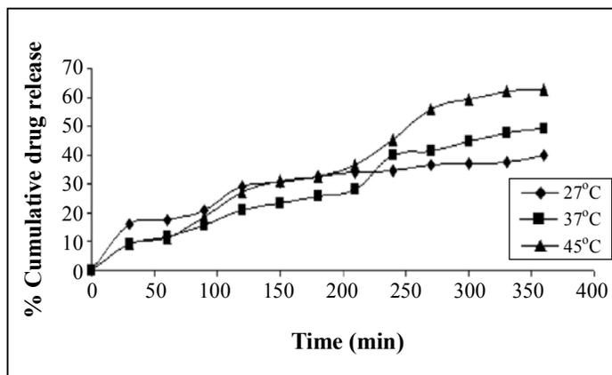
**Fig. 10: Release kinetics of cefixime from SMC beads at pH 1.2, different temperatures, shaking speed 80 rpm**
