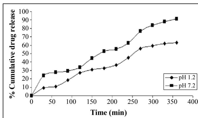
**Fig. 9:** *In vitro* cefixime release profile from SCMC beads at different pH, shaking speed 80 rpm at 45°C
