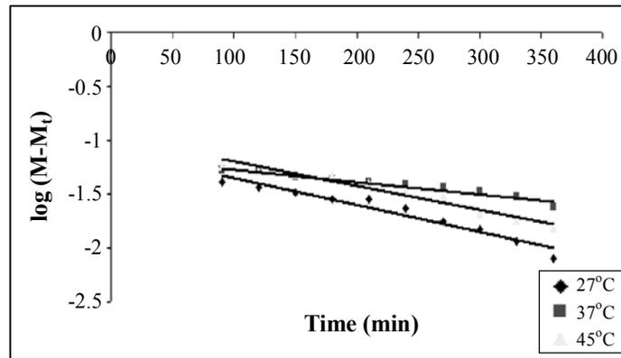
**Fig. 14: Plot of  $\log (M_{\infty} - M_t)$  vs. time of release of Cefixime from SCMC beads at pH 1.2, different temperatures, and shaking 80 rpm**
