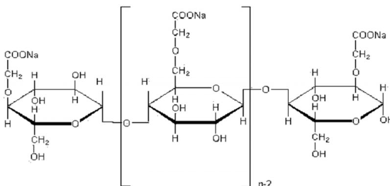
**Fig. 1: The chemical structure of sodium carboxymethyl cellulose<sup>9</sup>**
