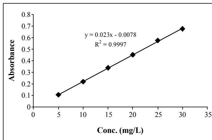
**Fig. 3: Calibration curve of cefixime by UV-Vis absorbance at 285 nm**
