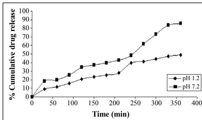
**Fig. 8:** *In vitro* cefixime release from SCMC beads at different pH, shaking speed 80 at 37°C
