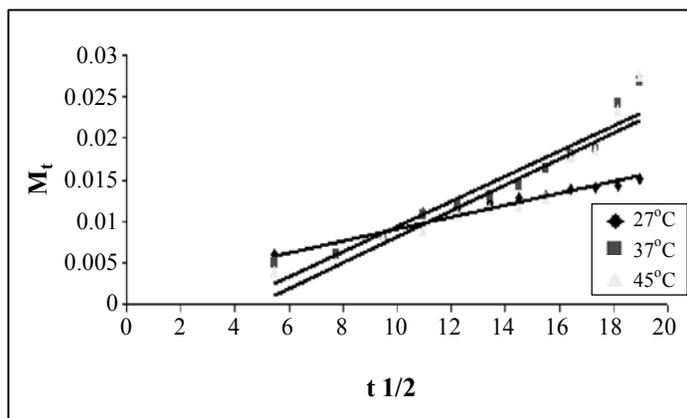
**Fig. 17:** Plot of  $M_t$  vs.  $t^{1/2}$  release of Cefixime from SCMC beads at pH 7.2, different temperatures, and shaking speed 80 rpm
