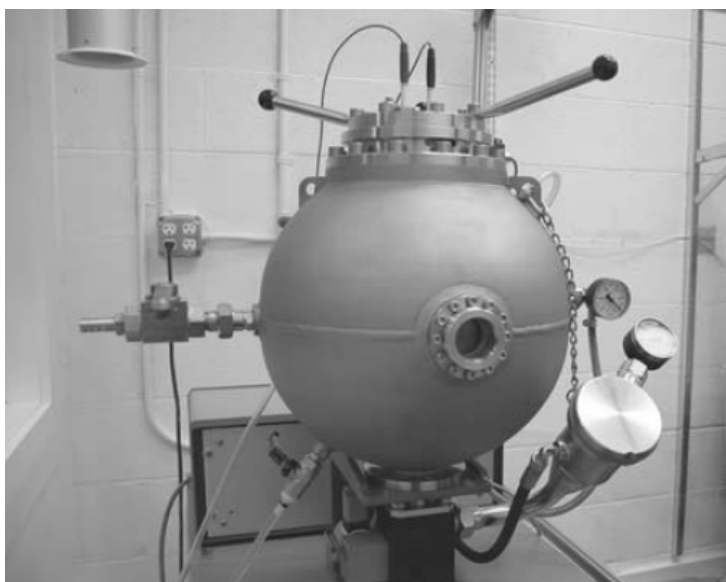
Fig. 2: 20-L-Apparatus for determining flammability characteristics of MPC 13, 14
