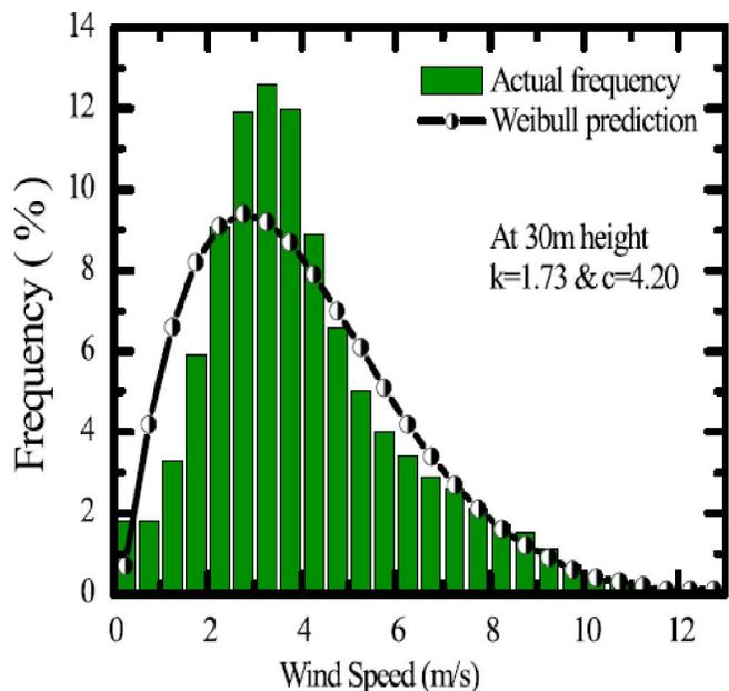
Figure 3 : Comparison between the actual frequency and Weibull prediction for wind speed at 30m height at Kuakata.
