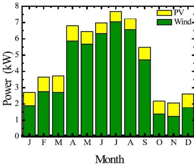
Figure 11 : Monthly average electricity production by PV and wind.
