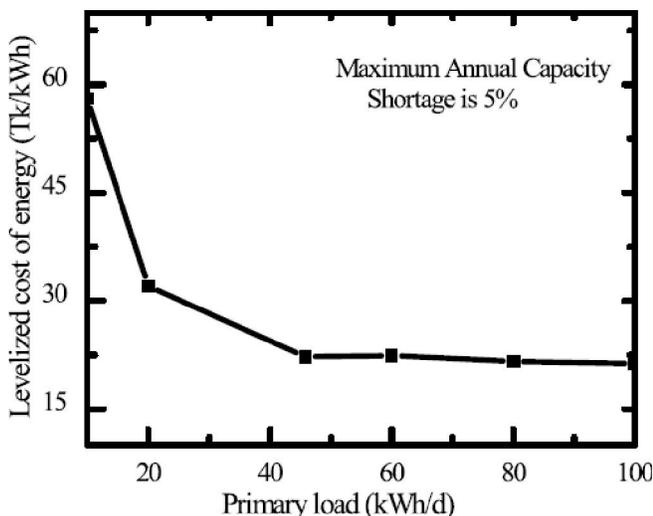
Figure 8 : The effect of primary load on LCOE.
