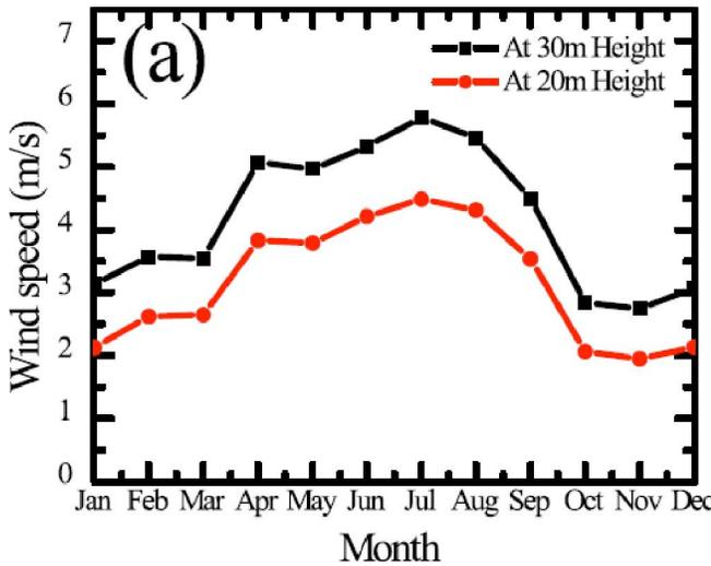
Figure 2 : (a) Monthly variation of wind speed of Kuakata at 30m and 20m elevation from the ground.
