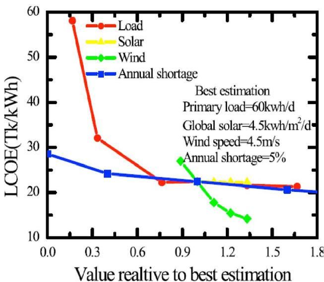
Figure 14 : Sensitivity of LCOE on solar radiation and wind speed.
