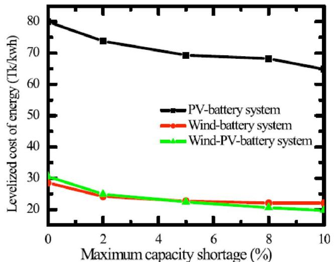
**Figure 7 : The effect of maximum annual capacity shortage on LCOE.**
