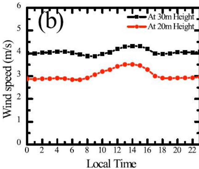
Figure 2 : (b) Hourly variation of wind speed of Kuakata at 30m and 20m elevation from the ground.
