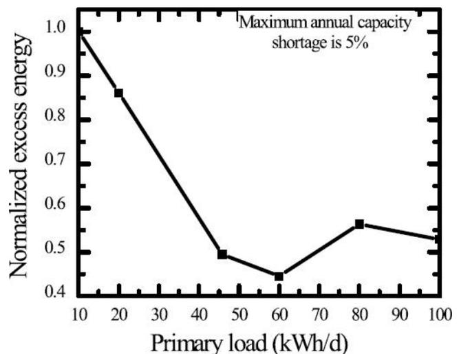
Figure 9 : The effect of primary load on normalized excess energy.
