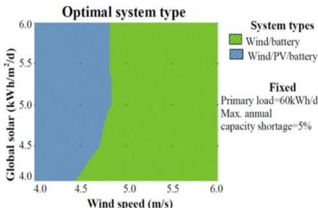
Figure 13 : Optimized hybrid system for 60 kWh/d load and maximum 5% annual capacity shortage.
