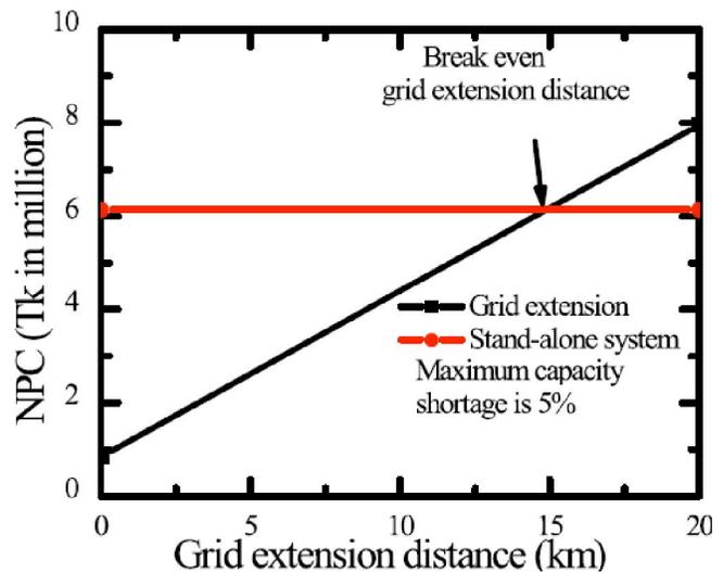
Figure 12 : Electrification cost for the grid extension and a standalone hybrid system.
