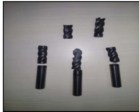
Fig. 5: Broken chatter free end mill cutter
