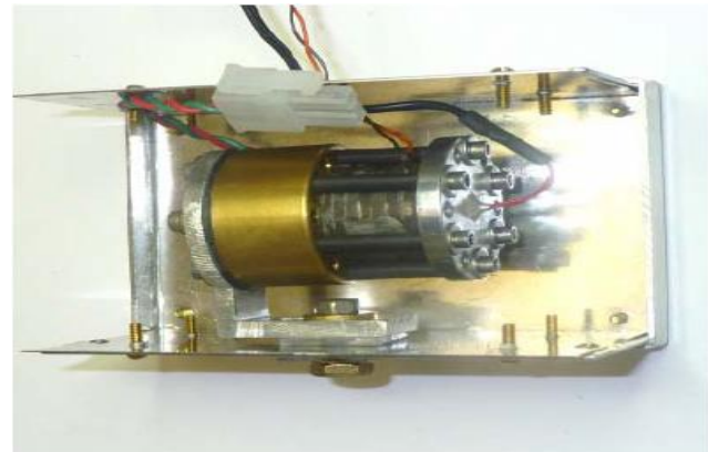
Figure 1 : A PZT stack device mounted in half of a Faraday cage. The Faraday cage sits on the end of a very sensitive torsion balance beam. Visible are the brass disc, the six 2-56 bolts covered with heat shrink for insulation, the PZT discs and aluminium end cap with embedded thermistor.
