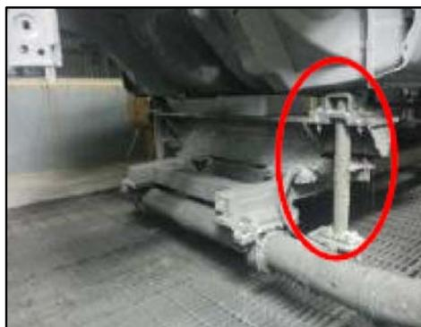
**Fig. 7: Locking mechanism with paint deposition**
