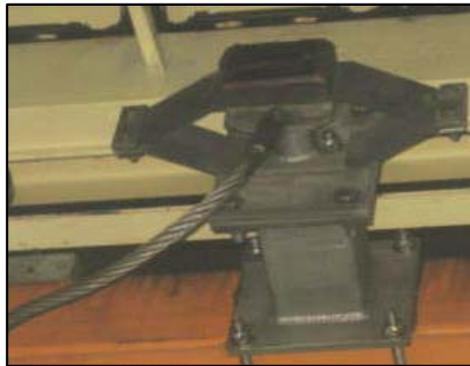
**Fig. 9: Cathode connection**
