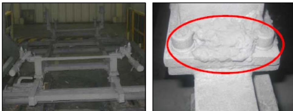
**Fig. 6: ED Coating in seating arrangements**
