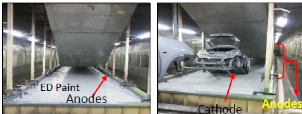
**Fig. 2: Typical ED bath of automobile industry**
