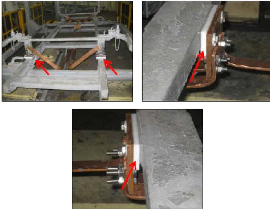
**Fig. 12: Insulators fixed on hangar to cathode connection**
