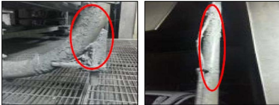
**Fig. 8: Excess ED coating on hangar surface**
