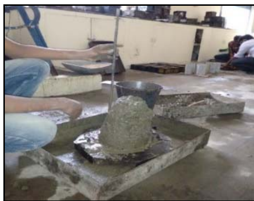
Fig. 3: Slump of RFRC
