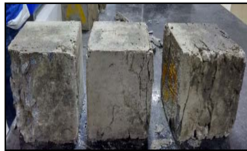
Fig. 5: 0.5% RFRC after testing
