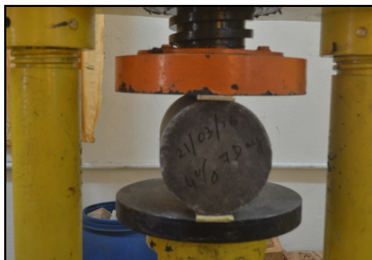
Fig.3.2 Split tensile test in CTM
