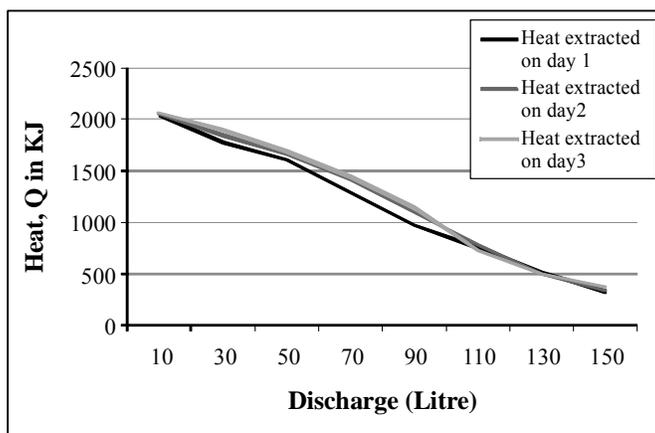
**Fig. 1: Heat discharge curve of thermal storage tank without PCM**
