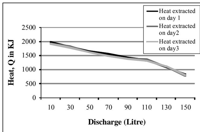
**Fig. 2: Heat discharge curve of thermal storage tank with PCM**
