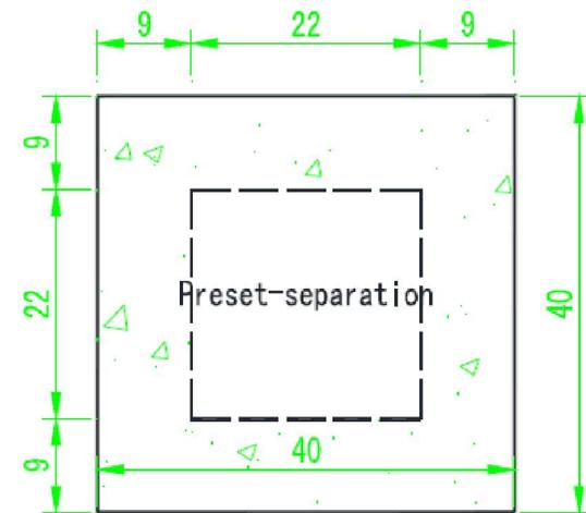
**Figure 3 : Layout of specimen 1: intact [unit: cm]**
