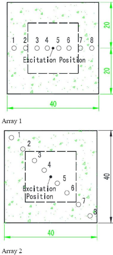
Figure 6 : Accelerometer arrays in Step 2 (The number represents the sequence of accelerometers)
