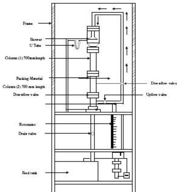
Figure 1 : Anaerobic fluidized bed reactor
