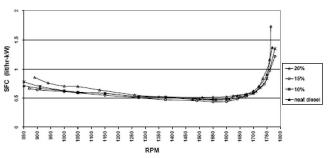
Figure 2 : Specific fuel consumption using emulsified fuels and neat diesel
