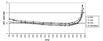
Figure 3 : Pure specific fuel consumption using emulsified fuels and neat diesel
