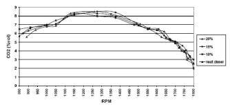
Figure 5 : CO<sub>2</sub> emission of neat diesel and emulsified fuels
