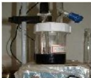
Figure 1: A two in one cell set up for potentiometric and titrimetric analysis
