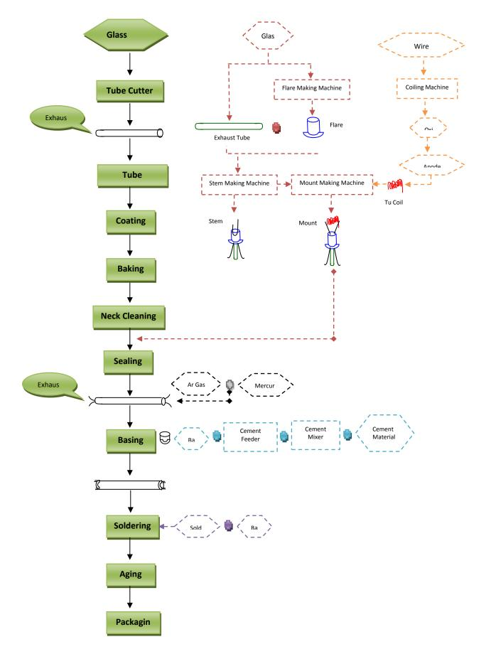
FIG. 2. Schematic representation of fluorescent tube light manufacturing procedures.
