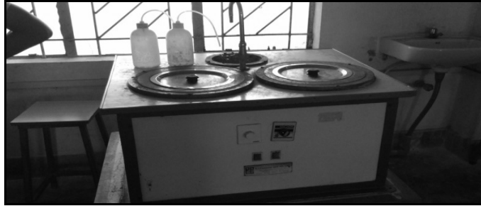
Fig. 3: Disc polishing to remove the coatings on the metal surface
