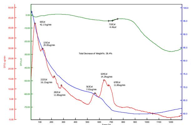
**Figure 2 :** Simultaneous thermal analysis (TG and DTA) of the dried powder. Data Name: NO:1.tgd, Module: TG/DTA, Sample name: dr hosseini, Sample weight: 1.740 mg, Reference name: empty pan, Reference weight: 0.000 mg. Comment:- Operator: icpc, Gas 1: none, Gas 2: Air, Pan: alumina. Temperature program:- Cel Cel Cel/min min s 1\*30 1300 15 0 0.5
