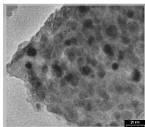
Figure 4 : TEM Micrographs of the fired powders at 1100°C/3h
