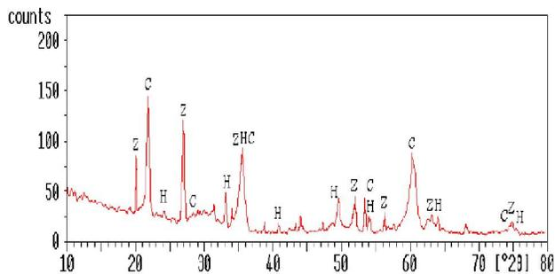
Figure 3 : XRD patterns of a) dried powder b) fired sample after calcination in 1000°C, H: Hematite, C: Cristobalite, Z: Zircon
