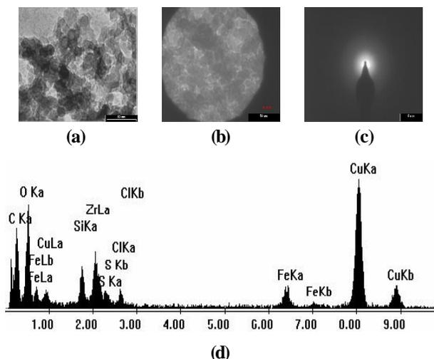
**Figure 1 :** TEM Micrographs of the dried powders and its EDX a) image, b) selected area diffraction zone, c) X ray pattern of it that indicates amorphous powder and d) EDX
