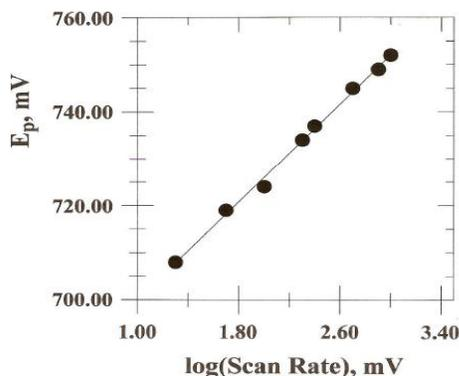
Figure 6 : The plot of the observed peak potential versus the logarithm of scan rate for 5.0mM congo red
