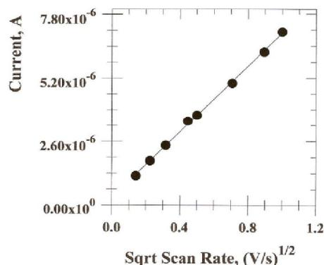
Figure 7 : The plot of the observed current versus the square root of scan rate for 5.0mM congo red
