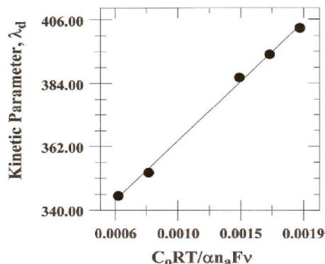
Figure 8 : Plot of the kinetic parameter versus the initial concentration times the time frame of the voltammetry of congo red for the determination of  $k_2$
