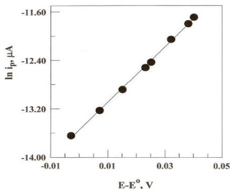
Figure 5 : Plot of the Ln of the observed current versus the observed peak potential minus the determined redox potential
