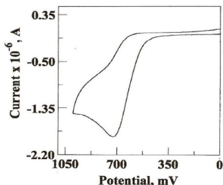
Figure 2 : The voltammogram of 5.0mM congo red at scan rate of 50.0mV/s
