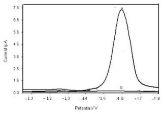
Figure 1 : Differential pulse stripping voltammogram of Mevinphos (a) at pH 2.0. Concentration: 0.01 mM, Deposition time: 30 sec., Pulse amplitude: 50 mV and blank solution (b)
