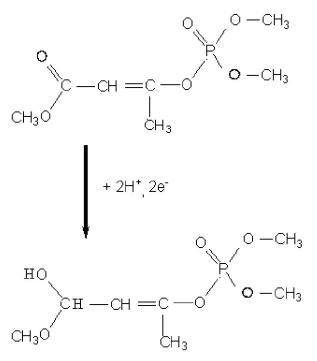
Scheme 2: Electrode reduction mechanism of mevinphos
