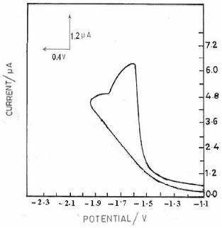
Figure 2 : Cyclic voltammogram of mevinphos at pH 2.0; concentration: 0.01 mM; scan rate: 50mVs<sup>-1</sup>
