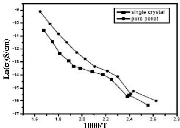
Figure 3 : Ln( $\sigma$ ) versus reciprocal temperature for CsNO<sub>3</sub>
