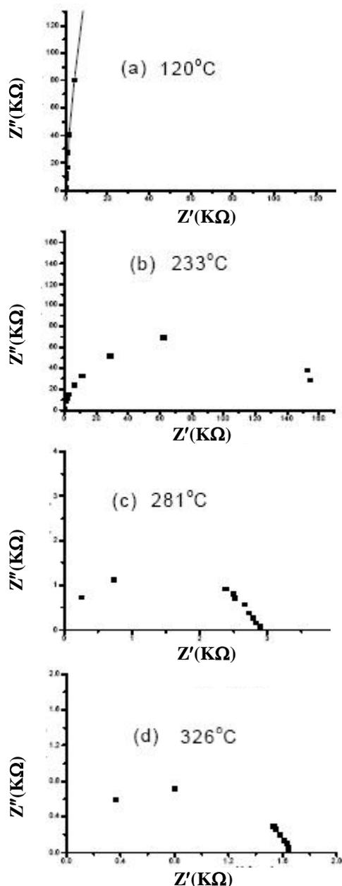
Figure 1 : Complex impedance plots for single crystal of  $\text{CsNO}_3$  at different temperatures
