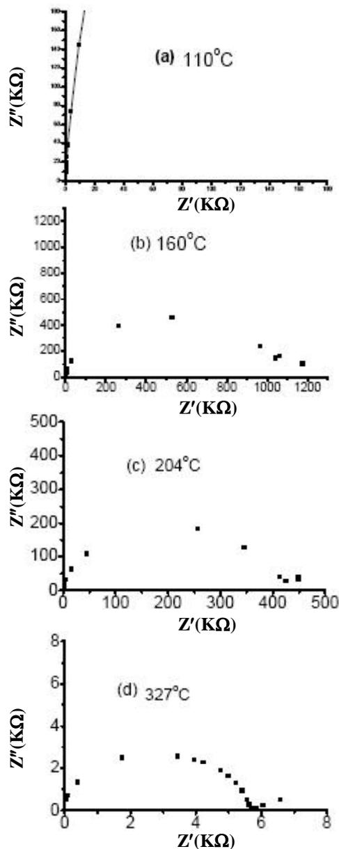
Figure 2 : Complex impedance Plots for pure  $\text{CsNO}_3$  pellets
