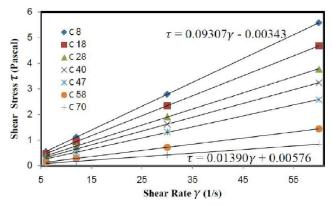
Figure 3: Relationship between shear stress and shear rate for olive oil sample from  $\mathbf{L}_1$  (2 year storage age) at different temperatures.
