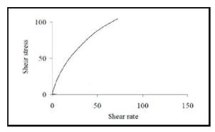
Figure 2: Flow curve of a Non - Newtonian fluid at power law Newtonian behavior. The greater the departure from
