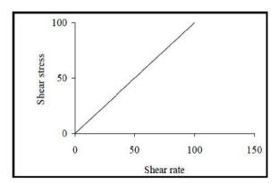
Figure 1 : Flow curve of a Newtonian fluid at power law basis for classical fluid mechanics. Gases, for example, exhibit characteristics of Newtonian viscos-
