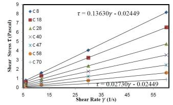
Figure 3: Relationship between shear stress and shear rate for olive oil sample from  $L_1(2 \text{ year storage age})$  at different temperatures
