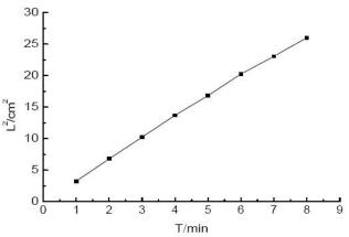
Figure 1 : L<sup>2</sup>-t relationship of carbon tetrachloride on silica column ( $\rho$ = 0.9935)
