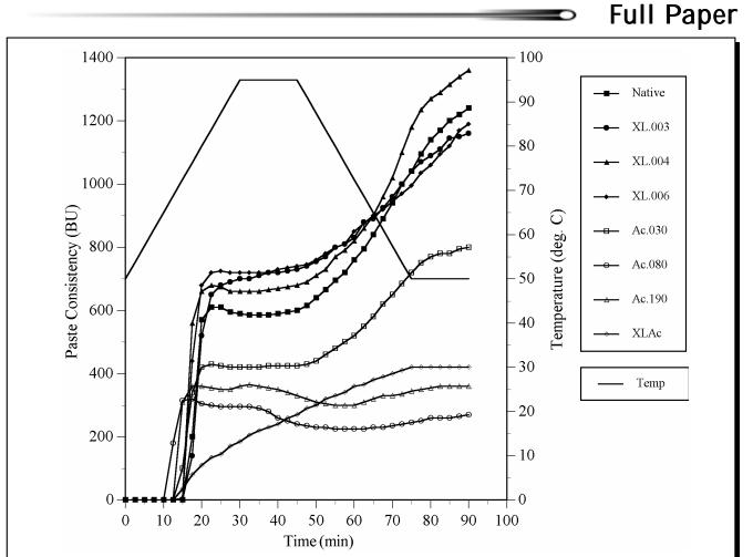
Figure 1: Effects of cross-linking (XL), acetylation (Ac), and double modification (XLAc) on the Brabender pasting profiles of cowpea starch. (In the legend frame, the numbers after XL and Ac denote the degree of substitution).
