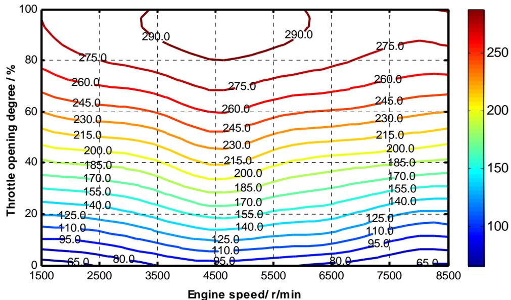
Note: The values marked in the figure represent NO<sub>x</sub> emission (10<sup>-6</sup>).
