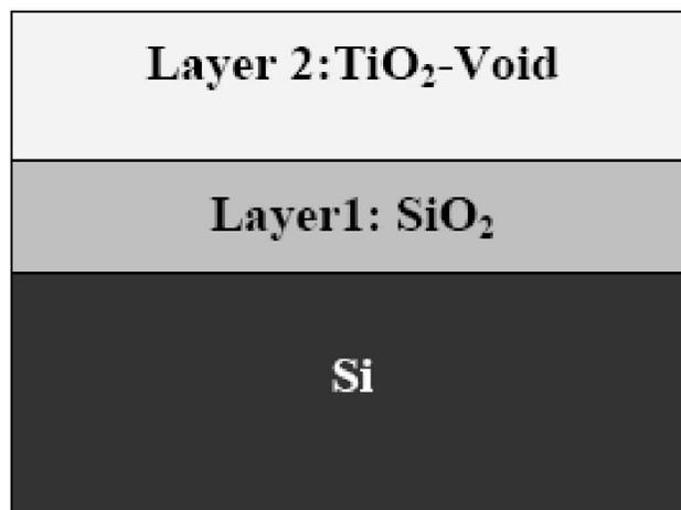
Figure 5 : The multilayer model of the  $\text{TiO}_2$  thin film on Si Substrate prepared by sol-gel method
