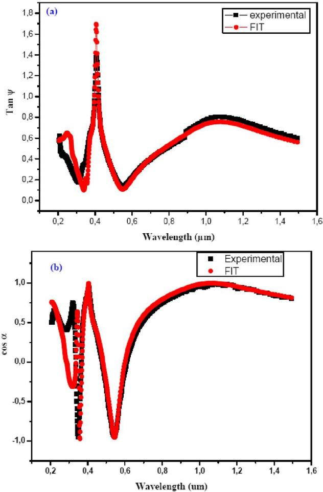
**Figure 6 : Ellipsometric measurement (Scatters) and modelling (lines), in terms of (a)  $\tan \psi$  and (b)  $\cos \Delta$ , as a function of wavelength, for TiO<sub>2</sub> annealed at 800°C in air for 1 h**
