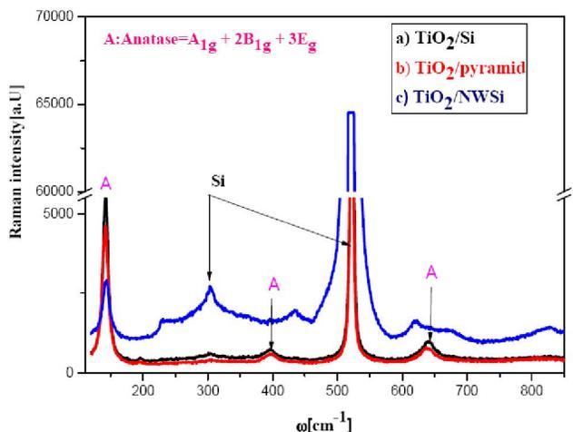
Figure 4 : Raman spectra of the (a)  $\text{TiO}_2/\text{Si}_p$ , (b)  $\text{TiO}_2/\text{Si}$ -pyramid and (c)  $\text{TiO}_2/\text{SiNWs}$
