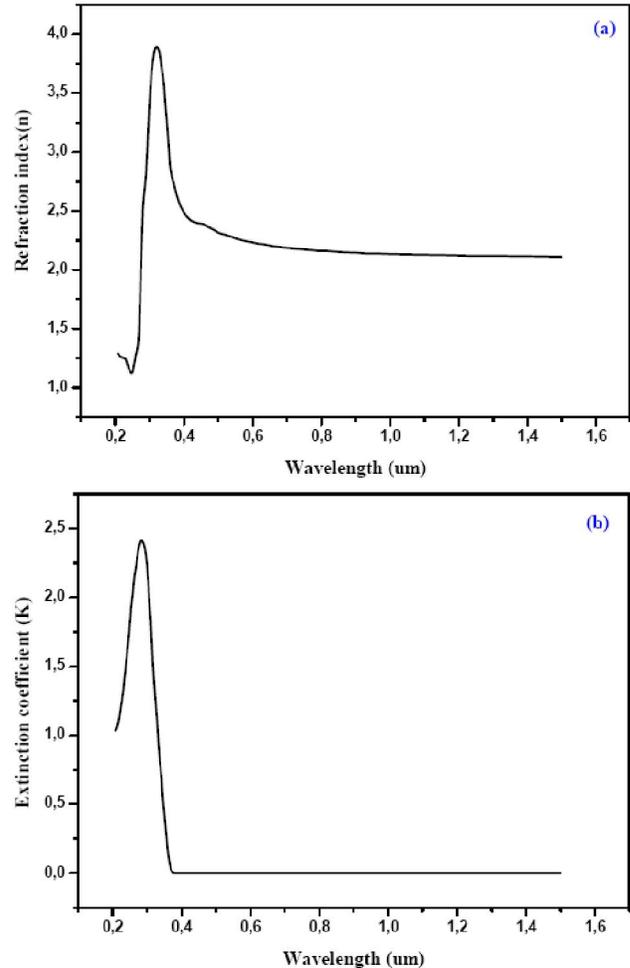
**Figure 7 : Refractive index (a) and extinction coefficient (b) as a function of wavelength of Titanium dioxide (TiO<sub>2</sub>) anatase phase**
