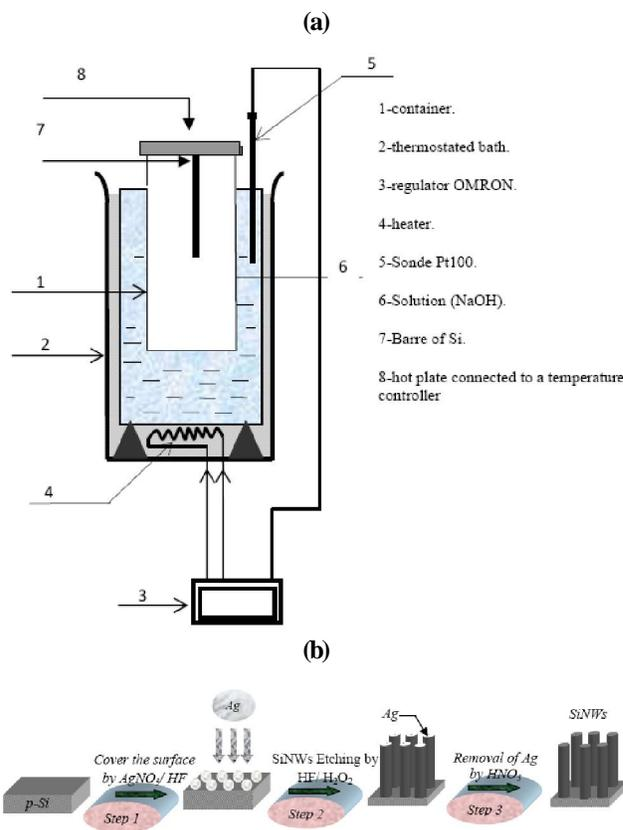
Figure 1 : Silicon nanowires growth mechanism
