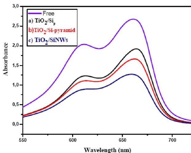
Figure 9 : Variation of the dye absorption spectra using  $\text{TiO}_2$  thin films deposited by sol-gel on various substrates on the photocatalytic activity
