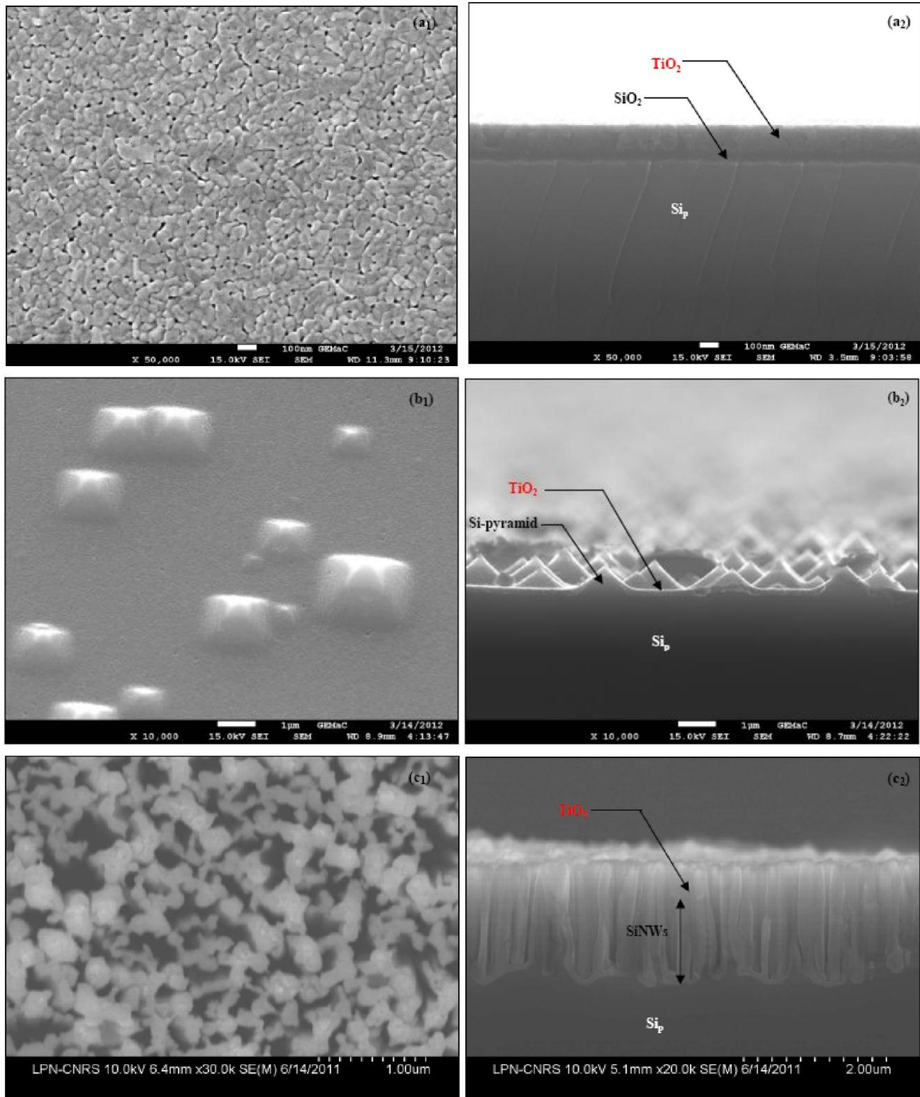
Figure 2 : SEM surface and cross section images of (a<sub>1</sub>,a<sub>2</sub>) TiO<sub>2</sub>/Si<sub>p</sub>, (b<sub>1</sub>,b<sub>2</sub>) TiO<sub>2</sub>/Si-pyramid and (c<sub>1</sub>,c<sub>2</sub>) and TiO<sub>2</sub>/SiNWs obtained by chemical etching technique and sol gel method
