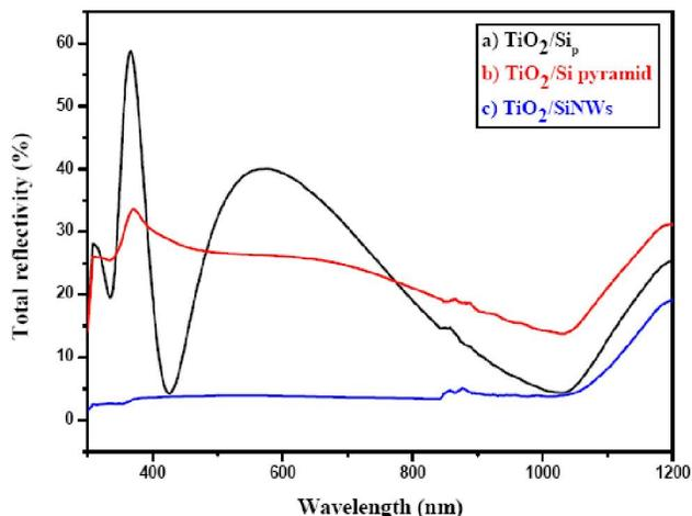
Figure 3 : Dependence of the total reflectivity of (a) Si-pyramid and (c) SiNWs before and after depot of  $\text{TiO}_2$  thin films. The reference corresponds to the bare substrate
