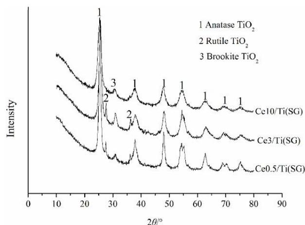
Figure 6 : XRD pattern of  $\text{CeO}_2/\text{TiO}_2$  catalysts prepared by SG method
