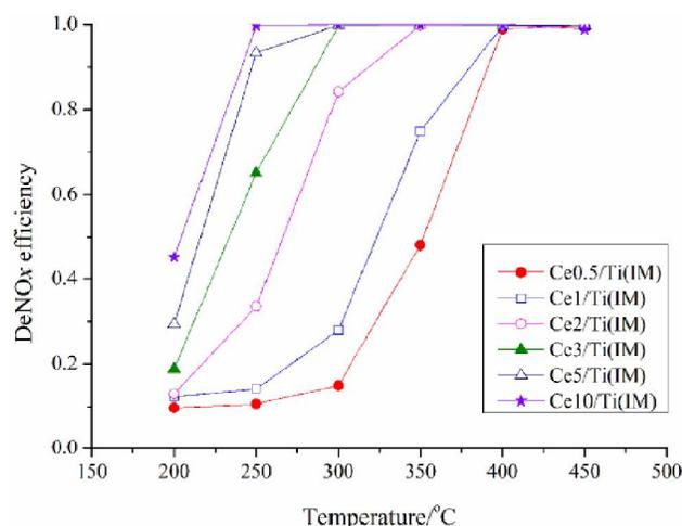
Figure 3 : DeNO<sub>x</sub> efficiency of  $\text{CeO}_2/\text{TiO}_2$  catalyst prepared by IM method
