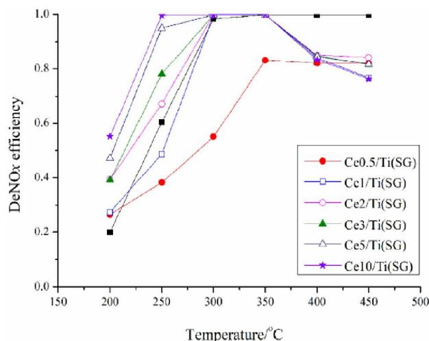
Figure 4 : DeNO<sub>x</sub> efficiency of  $\text{CeO}_2/\text{TiO}_2$  catalyst prepared by SG method
