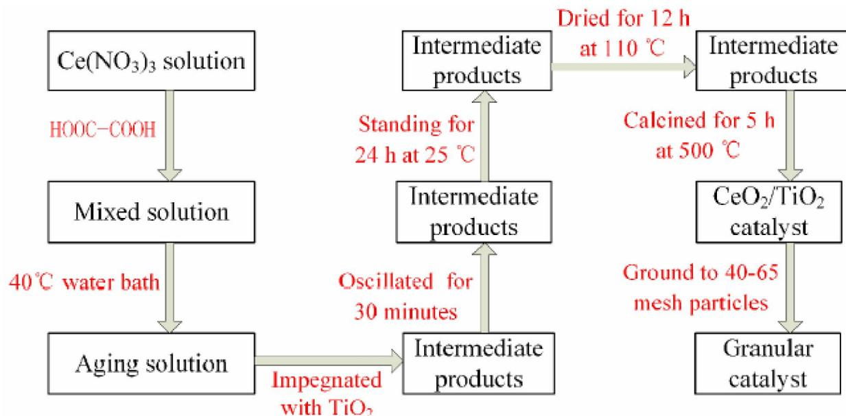
Figure 2 : Preparation process of granular  $\text{CeO}_2/\text{TiO}_2$  catalysts by IM method
