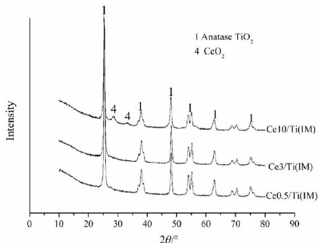
Figure 5 : XRD pattern of  $\text{CeO}_2/\text{TiO}_2$  catalysts prepared by IM method
