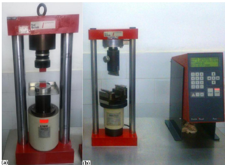
Figure 2 : Scheme of: a) compressive strength and b) flexural strength device
