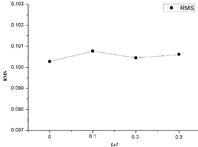
Figure 7 : RMS values of  $Le1$  of guiding plates in the turning
