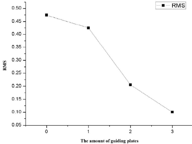
Figure 3 : RMS values of different amount of guiding plates in the turning
