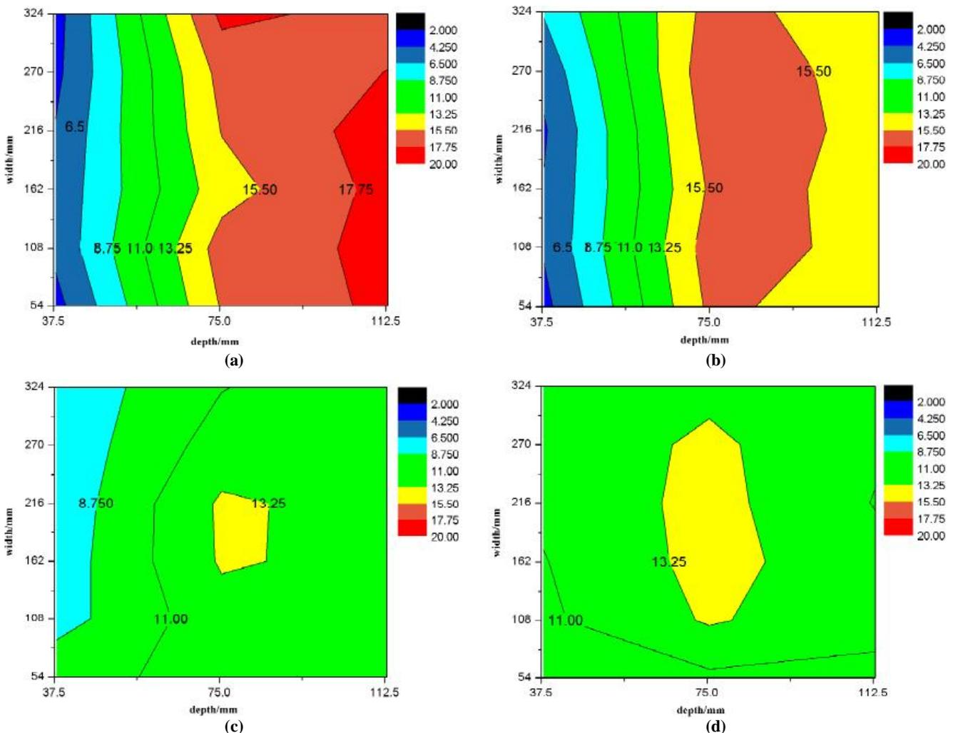
Figure 2 : IsovLOCITY graphs of different amount of guiding plates in the turning (a) 0 guiding plate; (b) 1 guiding plate; (c) 2 guiding plates; (d) 3 guiding plates
