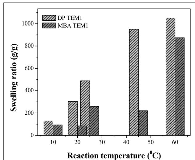
Figure 15: Influence of reaction temperature on swelling behaviour of crosslinked poly(AAm-co-SMA) copolymers
