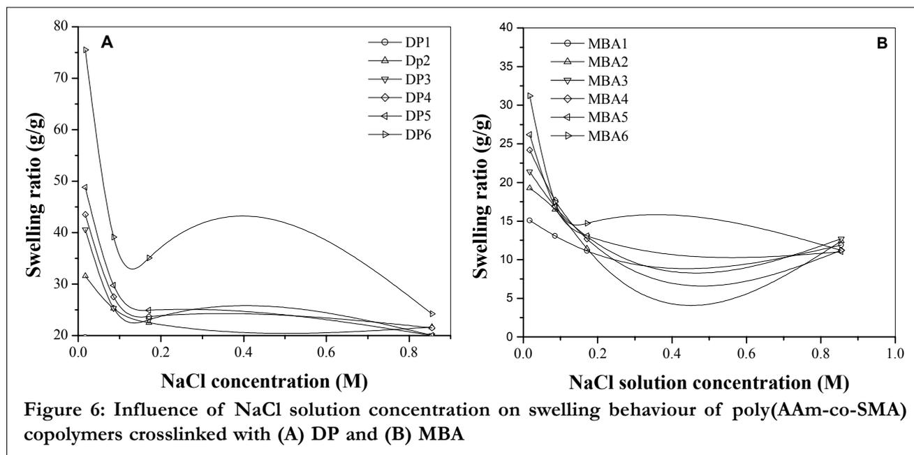
Figure 6: Influence of NaCl solution concentration on swelling behaviour of poly(AAm-co-SMA) copolymers crosslinked with (A) DP and (B) MBA
