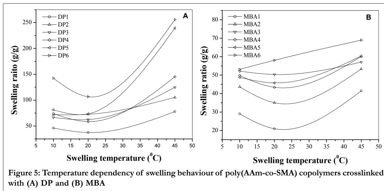
Figure 5: Temperature dependency of swelling behaviour of poly(AAm-co-SMA) copolymers crosslinked with (A) DP and (B) MBA
