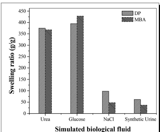
Figure 14: Influence of simulated biological fluids on swelling behaviour of crosslinked poly(AAm-co-SMA) copolymers
