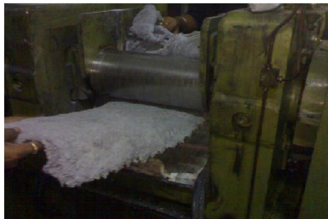
Figure 2 : SBR compound mixed on two roll mill
