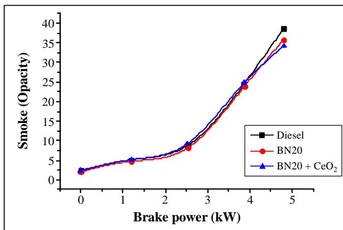
**Fig. 12: Variation of smoke emission with brake power**
