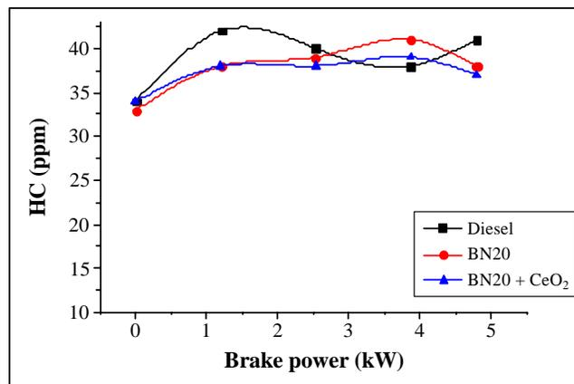
**Fig. 10: Variation of HC emission with brake power**
