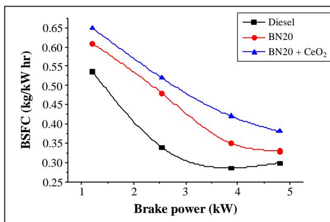
Fig. 5: Variation of BSFC with brake power
