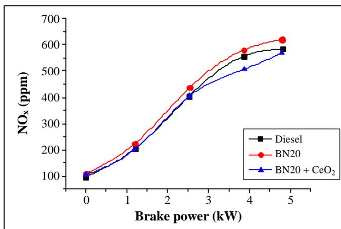
**Fig. 11: Variation of NO<sub>x</sub> emission with brake power**
