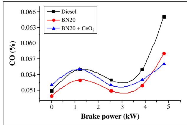
**Fig. 9: Variation of CO emission with brake power**
