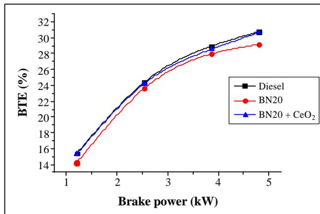
Fig. 6: Variation of BTE with brake power
