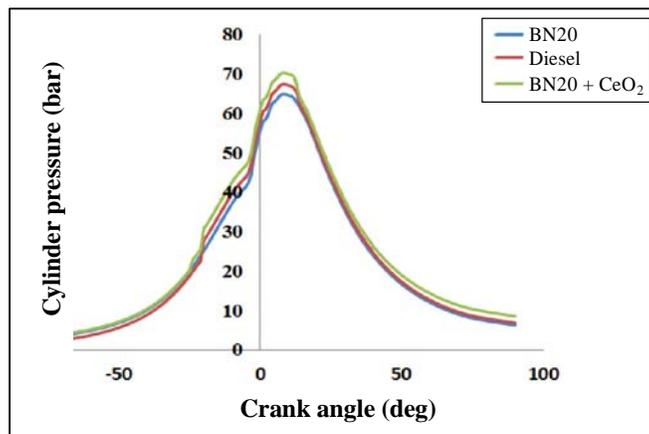
Fig. 7: Variation of cylinder pressure with crank angle
