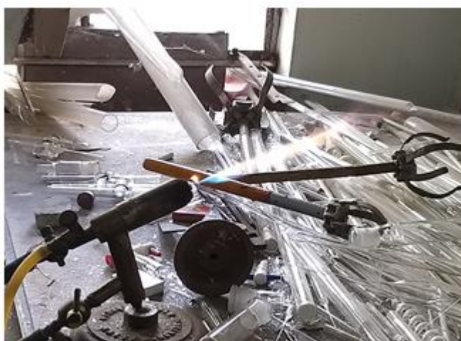
FIG. 3. Encapsulation through quartz glass blowing.
