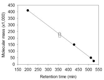
Figure 1 : Relative molecular weight of EPS determined by gel filtration chromatography. A standard dextran (Fluka, molecular mass, 25,000, 50,000, 150,000, 410,000) was used to calibrate the relationship between retention time and molecular mass (closed symbols). Molecular mass of EPS was determined by 4 times-repeated tests (open symbols).
