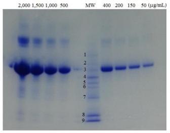
Figure 2 : SDS-PAGE image of solubilized human hair proteins (HHP) obtained by heat treatment under alkaline condition. Protein concentration of samples for electrophoresis was adjusted to 2,000~50 mg/mL to visualize bands of minor proteins and obtain clear band of major proteins. MW indicates protein markers that are separated based on molecular weight of standard proteins (1, 225,000; 2, 150,000; 3, 100,000; 4, 75,000; 5, 50,000; 6, 35,000; 7, 25,000; 8, 15,000; 9, 10,000)
