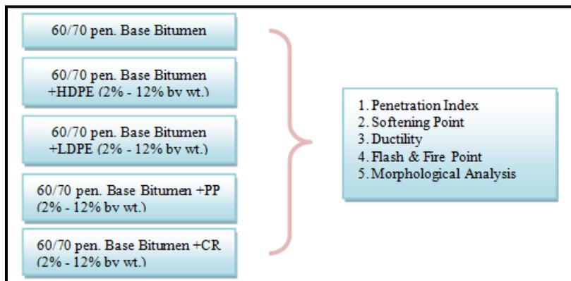
**Fig. 4: Methodology adopted for modification of 60/70 pen. Bitumen**
