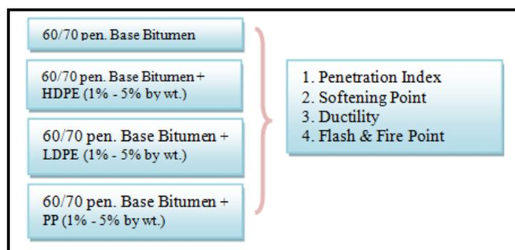
**Fig. 5: Methodology adopted for modification of 80/100 pen. Bitumen**
