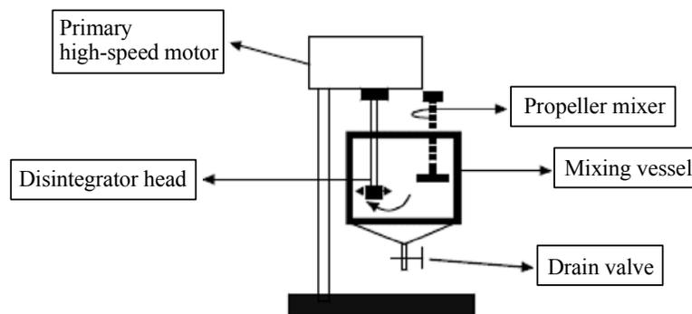
**Fig. 3: Polymer-bitumen mixing assembly**
