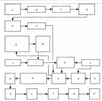
Note: A-coke gas washed; B-coke oil trap; C-get rid of acid; D-coke gas tank; E-coke gas compressed; F-desulfuration with wet process; G-hydrogenation; H-desulfuration with dry process; I-condensation; J-saturation tower; K-steam heat; L-overheating steam; M-residual heat recovery; N-convertor; O-boiler; P-oxygen and steam mixture; Q-oxygen; R-condensation and separation; S-compression; T-generate methanol; M-methanol's rectification; N-methanol's tank.
