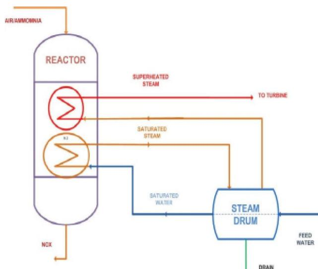
Figure 1 : Schematic diagram of WHB internally coupled in ammonia oxidation reactor
