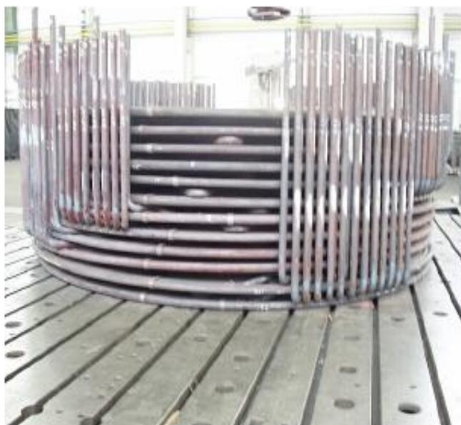
Figure 2 : Uninstalled connecting tubes of WHB.
