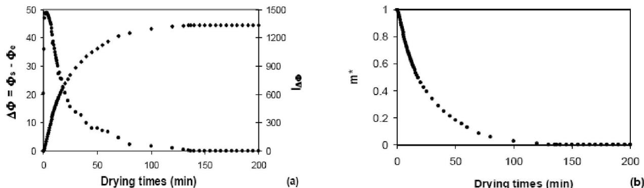
Figure 3 : (a) Integral under the curve of  $\Delta\Phi = f(t)$  and (b) standardized form of the integral,  $I\Delta\Phi$ , for a dry air flowrate of about 48 l/mn at ambient temperature
