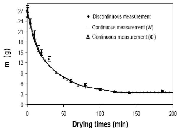
Figure 4 : Evolution of the mass of carrot particles versus time for a dry air flow-rate of about 48 l/min at ambient temperature
