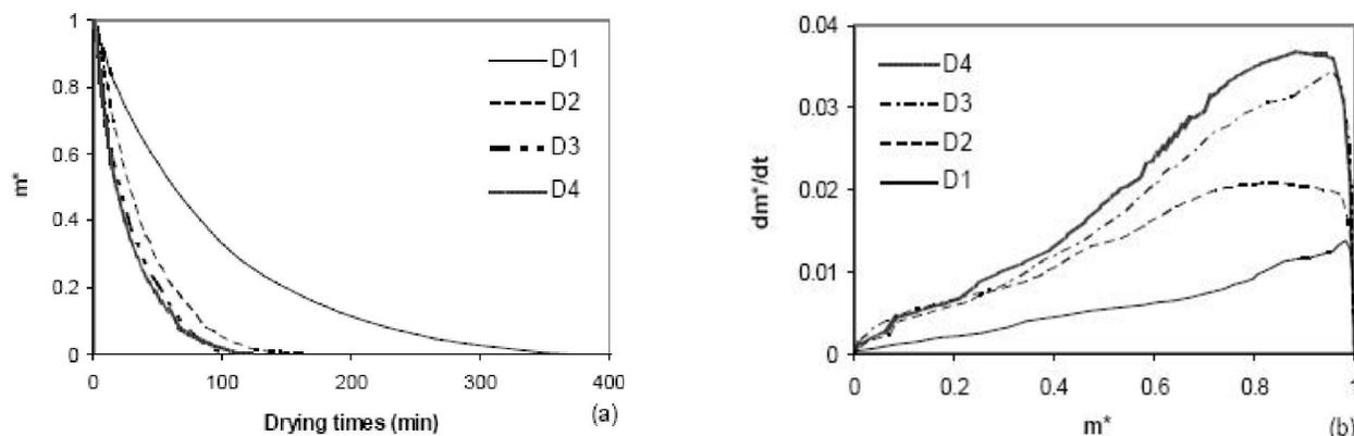
Figure 5 : Drying kinetics and rates of carrot gratings versus time at different dry air flowrate at  $T_{amb}$ ; D4 = 48 l/min, D3 = 38 l/min, D2 = 20 l/min and D1 = 10 l/min
