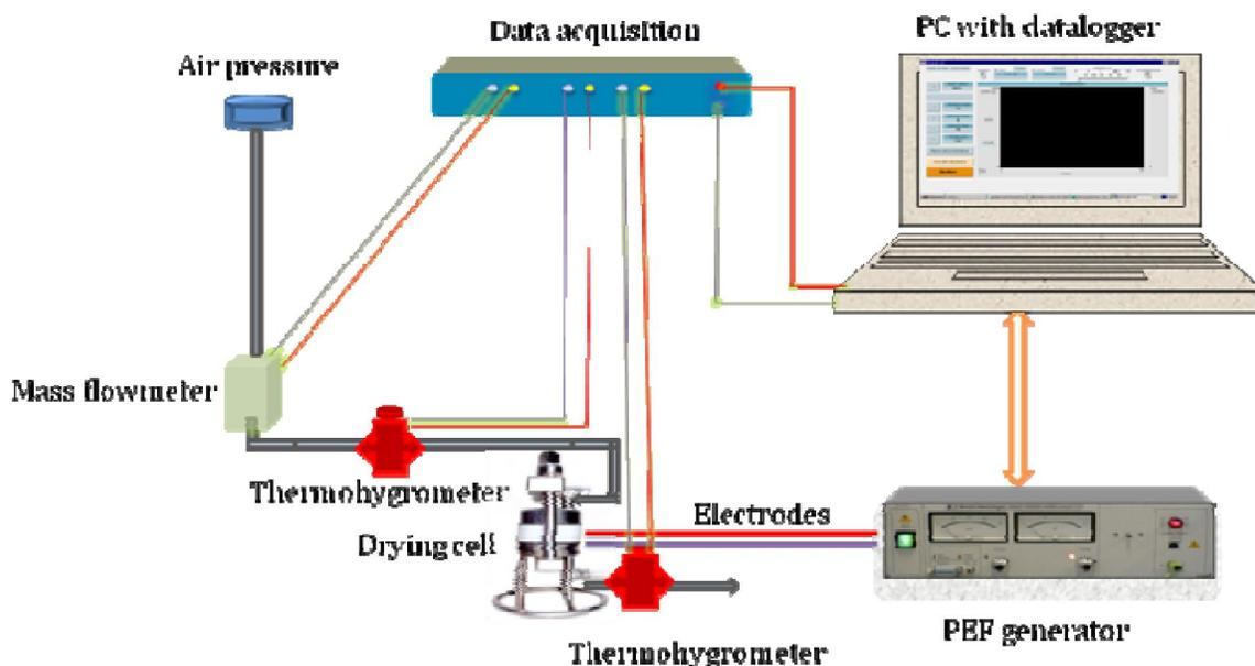
Figure 1 : Schematic of the experimental drying unit
