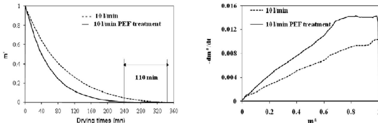
**Figure 7 :** PEF pre-treatment effect on drying kinetics and rates of carrot gratings at air flowrate of 10 l/min and ambient temperature: (...) untreated samples, (—) treated samples
