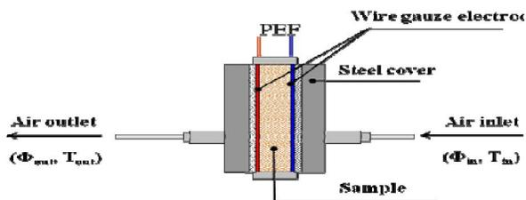
Figure 2 : Schematic of the drying cell
