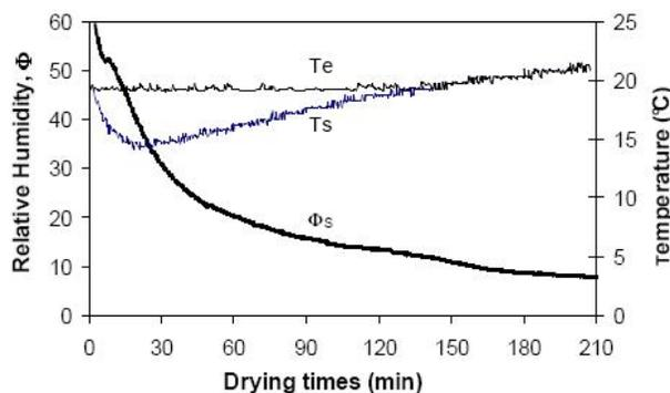
Figure 6 : Humidity and temperature evolution during drying of carrot gratings at air flowrate of 48 l/min
