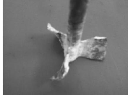
Figure 1 : The three blades stainless steel stirrer.
