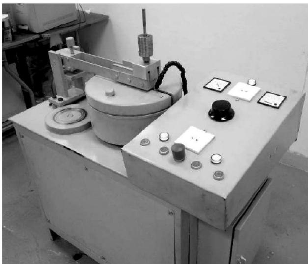
Figure 3 : The pin-on-disc wear tester.
