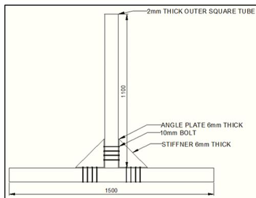
**Fig. 1: Beam-column connections**
